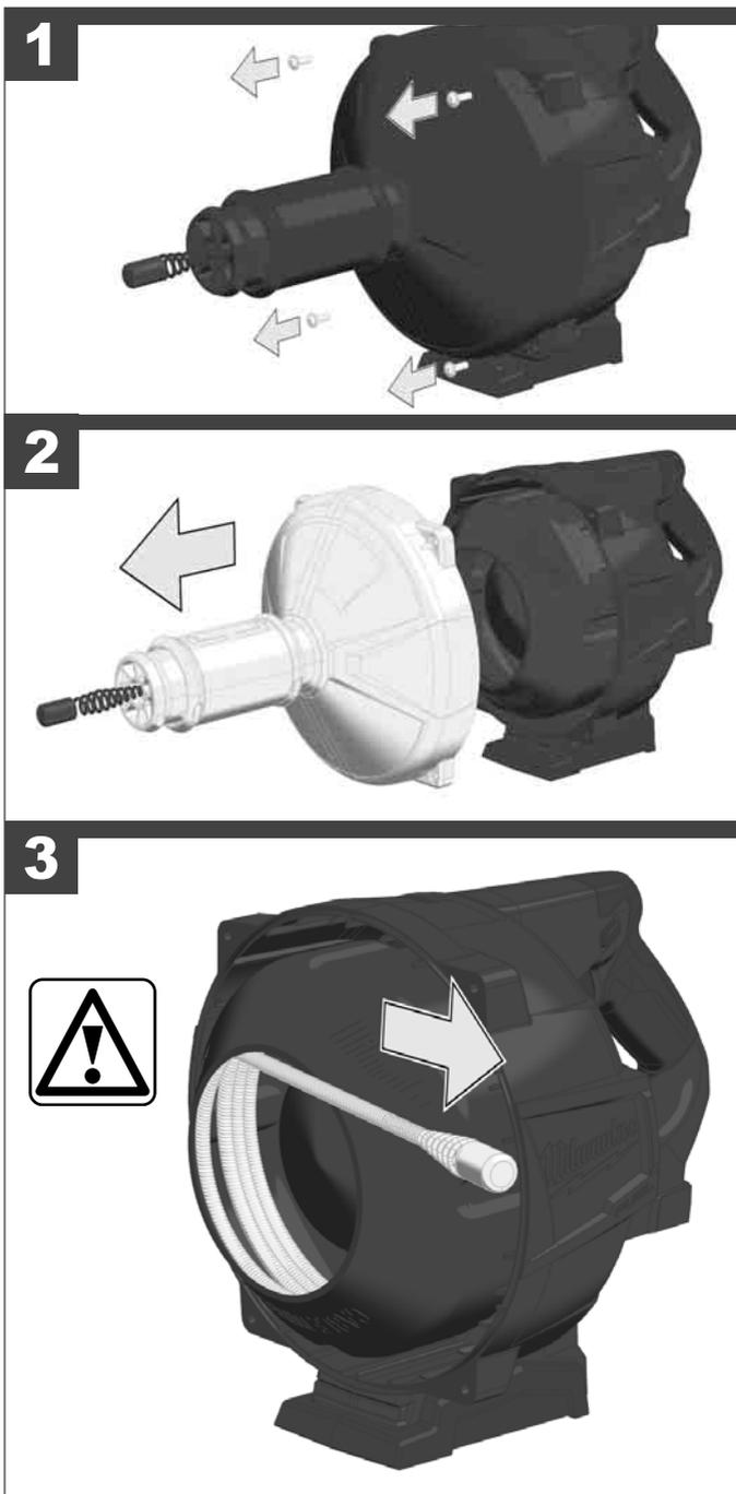
**Attention!** Cable is under high tension in the container. Remove cable carefully from the container.
