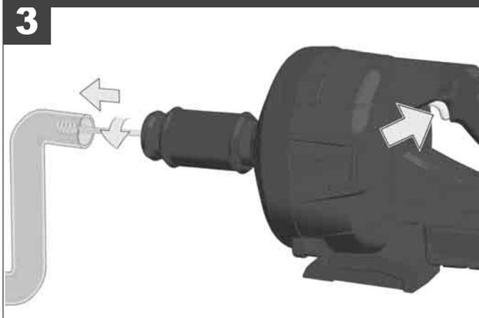
Switch on - cable rotates.
