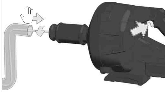
Switch on - cable rotates.
