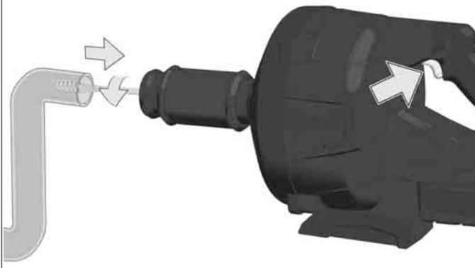
Switch on - cable rotates.
