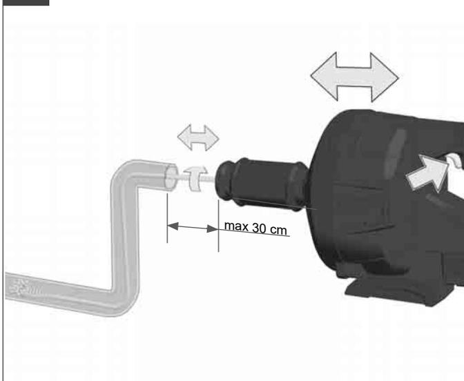
Switch on - cable rotates. Eventual change the direction of rotation or move machine back and forth.
